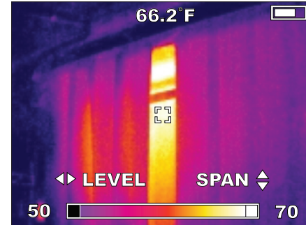
Figure 13. Setting Level and Span for Manual Range
