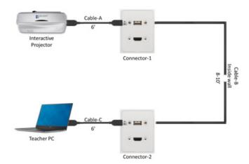
A common area where problems occur is when an interactive display device, usually a projector or flat panel, is mounted on the wall and cables run through the wall to connect to the teacher PC. Total cable runs in excess of 30', sometimes with multiple cables daisy chained, have been observed—well beyond any reasonable expectation of "do no harm" successful data connections. The example below shows approximately 22' of physical length that could easily be 25–30' of electrical length.
