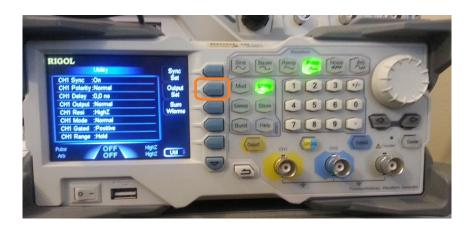
Now you can adjust the Amplitude High and Low values within a fixed range with minimal glitching.
