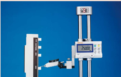
Checking accuracy of height gage
