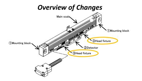
3 – Head Fixture change: Abolishes screwing to the scale body, allowing fixing and mounting at locations other than the center of the overall length.
