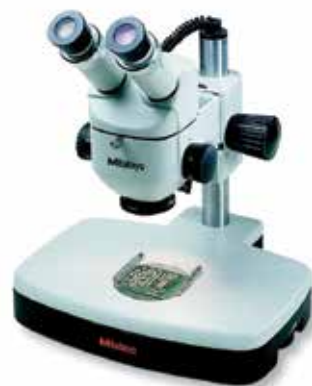
Stereo Microscope with Stepped-Magnification Lenses
