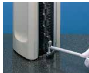
Using height master to set bore gage
