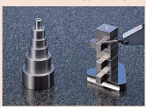
Using plain jaws, gauge blocks, a tie rod and a knurledhead screw a gage was constructed to enable rapid comparison measurement of a stepped workpiece. (Sample workpiece)
