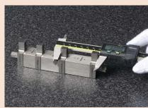
Using plain jaws, gauge blocks, a tie rod and a knurledhead screw a gage was constructed to enable rapid checking of the accuracy of a caliper at selected points.
