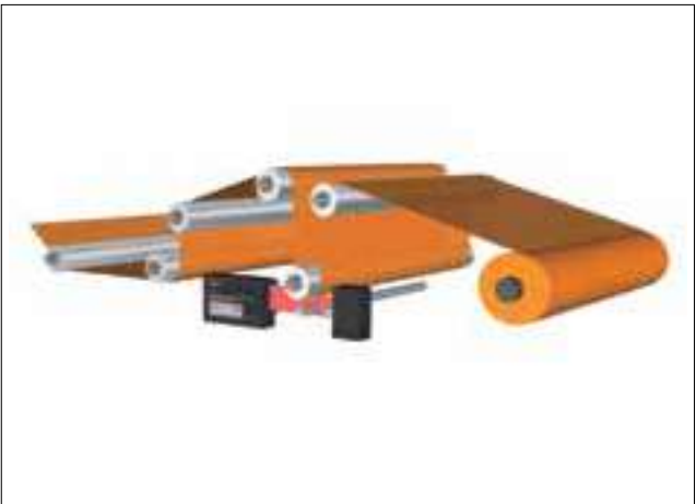
Measurement of film sheet thickness
