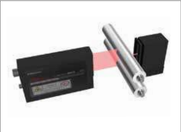
Measurement of gap between rollers
