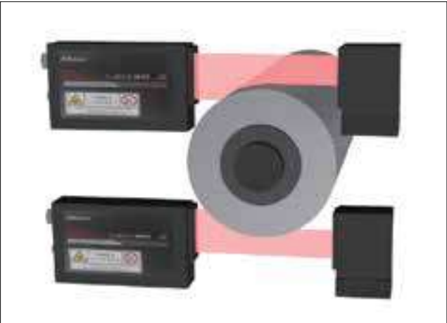
Dual system for measuring a large outside diameter
