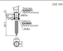
For 50 mm **LG100** Components Thrust stem: **02ADN371**
