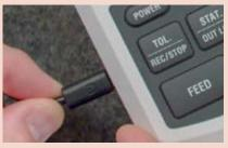
USB connection allows collected data to be easily transferred from the DP-1VA to the PC. The output is HID or VCP so data can be sent directly to Excel or data collection software such as IT-Pak or MeasurLink.
