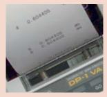
Digimatic 2 function allows the high resolution of the gage to be output in its entirety in metric or inch.
