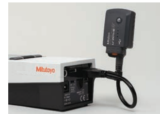
Example of the connection with SJ-210
