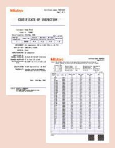
A Certificate of Accuracy, traceable to the NIST, is furnished with each gage block set and individual block.
