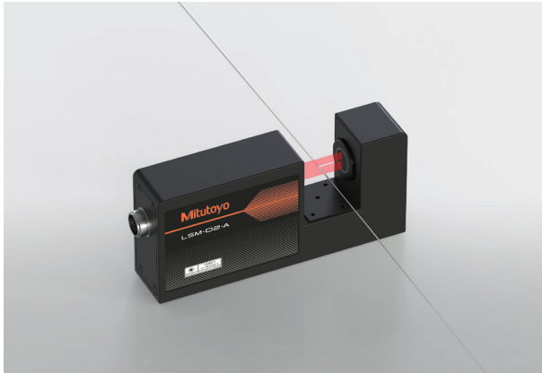
Simultaneous measurements of roller outer diameter and deflection
