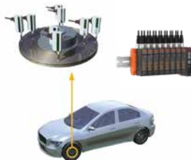
2 Brake disc multipoint measurement
