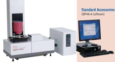
The GBCD-100A Automatic Gage Block Comparator is an easy-to-operate dualhead gage block inspecting system. It automatically compares workpieces with a standard gage block and determines accuracies such as central length, maximum length, minimum length and parallelism through the operation of an optional personal computer.
