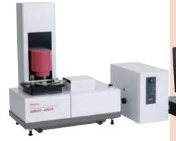
The GBCD-100A Automatic Gage Block Comparator is an easy-to-operate dualhead gage block inspecting system. It automatically compares workpieces with a standard gage block and determines accuracies such as central length, maximum length, minimum length and parallelism through the operation of an optional personal computer.
