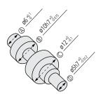
Measuring procedure: Measure the dimensions numbered (A) to (D), perform tolerance judgment, and statistically process the resulting data for every ten samples defined as one lot.
