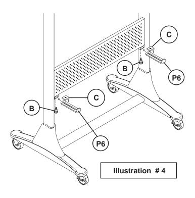
6.) Your Genius Stand is shipped with two Long Brackets(P6) installed at the top. You may need to change these brackets and use two Short Brackets(P5) if your board is thinner. See illustration #5.
