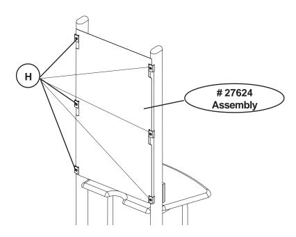
2.) Take the assembly from the end of Step #3 of the iTeach Electric Wall Mount (#27606) and hook the mount tabs that are the back frame into the six brackets that the Back Panel of # 27624 is hooked into. See Illustration # 2.
