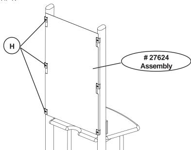
2.) Take the assembly from the end of Step #3 of the Elevation Wall Mount (#27589) and hook the mount tabs that are on the back frame into the six brackets that the Back Panel
