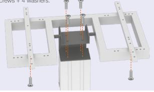
Make sure to run the two cables exiting the column through the cut out of the board frame before securing the 4 bolts.
