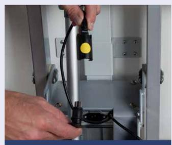
Put the plug of the external actuator into the connector marked with the yellow dot.
