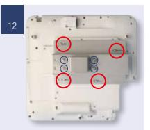
Carefully place the projector plate on top of the spacers and washers and secure the plate with 4 x allen head screws M4 x 20 (0.15" x 1 3/4").
