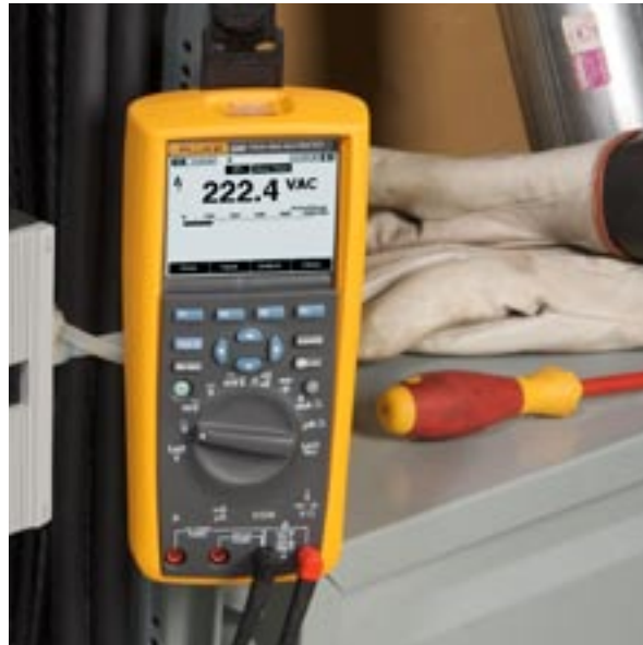
Output voltage reading with low pass filter enabled
