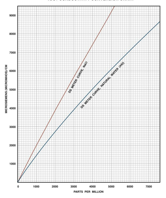
**Note:** The 442 to Conductivity correlation is non-linear and no single multiplier can be used to determine the relationship.
