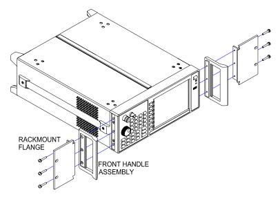
4 Rack mounting with two dress screws per side.
