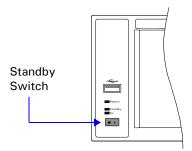
Pressing this front panel switch toggles power to the signal generator between on (green LED on) and standby (orange LED on). In standby mode, the signal generator is switched off, however the instrument is still connected to the line power. The rear panel line switch and the detachable power cord are the instrument disconnecting device. The front panel standby switch, therefore, is not, and should not be used as a power switch.
