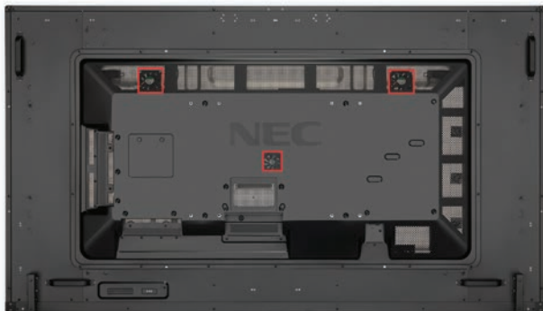
Location of Thermal Management Cooling Fans
