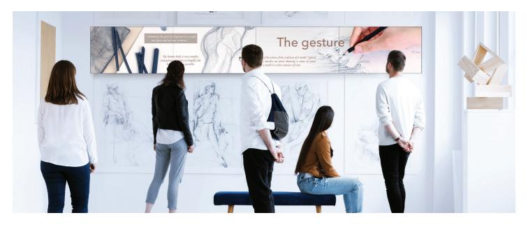
Selecting the best video wall solution for a specific indoor installation can be challenging. Here are some considerations to keep in mind: dvLED is capable of creating very high brightness levels of up to 5,000 cd/m<sup>2</sup> or more which is required for large scale outdoor screens, whereas indoor screens typically feature brightness levels of between 500 and 1,200 cd/m<sup>2</sup>.
