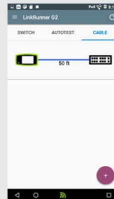
Distance to Open while connected to Switch
