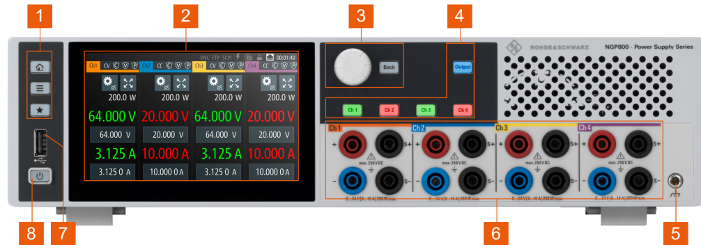
Figure 3-2: Front panel of R&S NGP800 power supply
