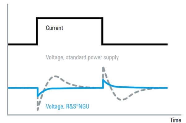
Under challenging load conditions, most power supplies respond with slow recovery times and overshoot. Specially developed circuits in the R&S®NGU source measure units achieve a load recovery time of < 30 µs with minimal overshoot, making them perfect for supplying sensitive components with power.
