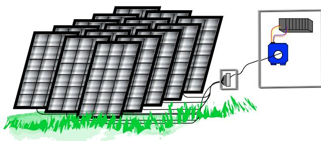
Commercial and industrial ground mounted solar arrays are connected in series to combiner boxes, developing higher voltage and lower current to deliver the same power as with a lower voltage system.
