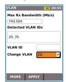
Automatic detection of VLAN ID's allows the user to configure NaviTEK NT for operation on a VLAN.
