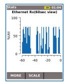
Real time display of broadcast network traffic shown as a percentage of port speed for the previous 60 minutes.
