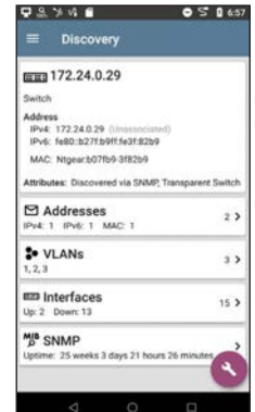
Device detail showing VLAN, interfaces, uptime, & more with drill-down
