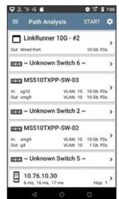
Path Analysis shows the device & interfaces that UDP/TCP traffic traverses
