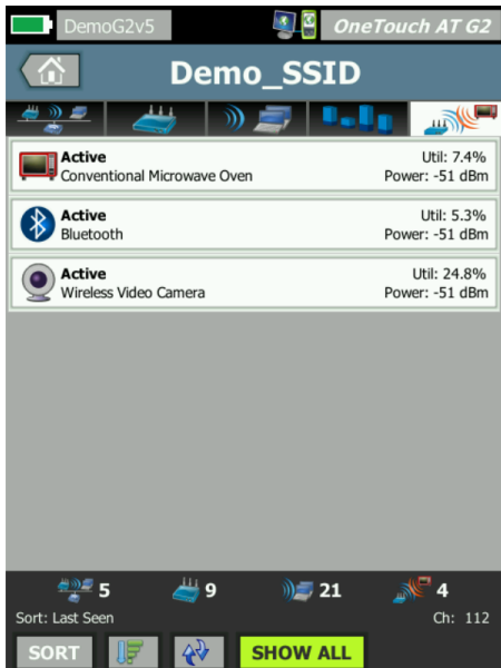
Figure 15. Unique Interferer analysis classifies sources of non-802.11
