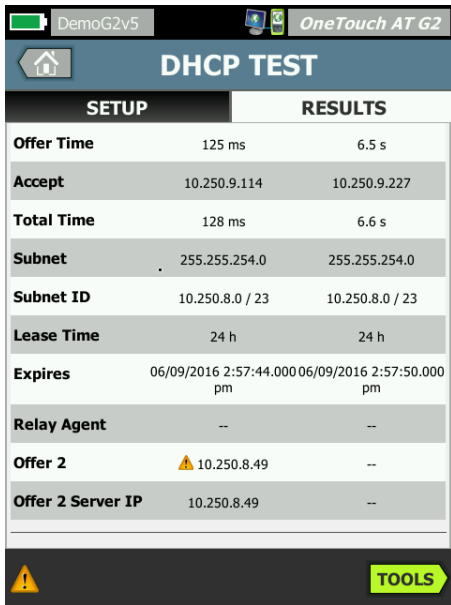
Figure 6. Detailed breakdown of DHCP provisioning and response performance
