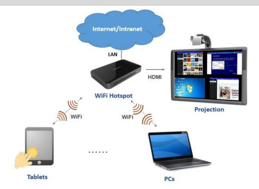
As described in Section 1.3, you can enable the routing between LAN and WiFi Hotspot. Once you enable this routing feature, devices on the WiFi Hotspot side will be able to access intranet or Internet resources via the LAN connection.
