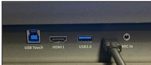
Front Ports with USB Type-C cable connected.
