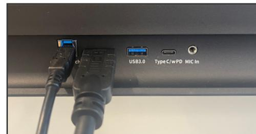
Front Ports with USB Type-B and HDMI cable connected.
