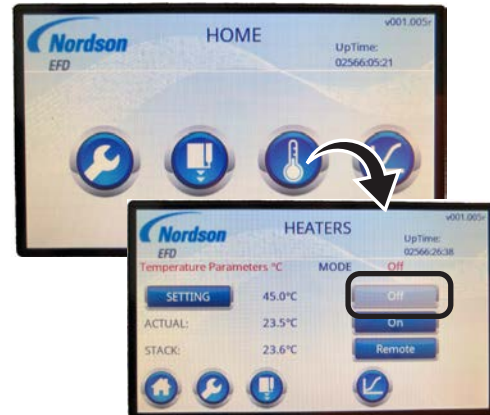
Switching OFF heater control
