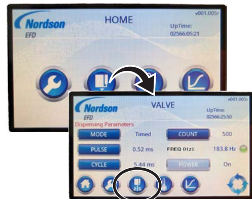
Location of the PURGE button (standard Touch controller VALVE screen shown)
