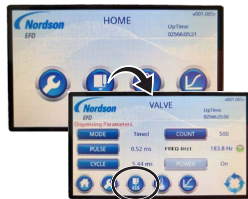
Location of the PURGE button (standard Touch controller VALVE screen shown)
