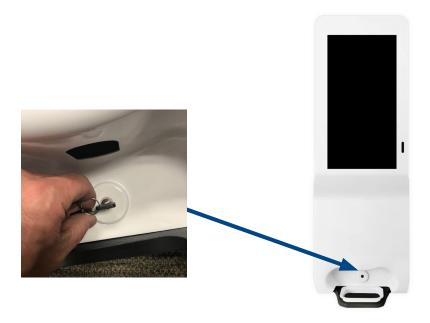
Remove the dispenser tank from inside the kiosk, there are no cords or electronics attached to the tank so you can remove in one piece with one tug. Unscrew the nozzle from the tank, then refill the tank with any liquid, gel or foam sanitizer. Reattach the nozzle to the tank then place the tank and nozzle assembly back into the kiosk. Close the white panel casing and lock with the key.
