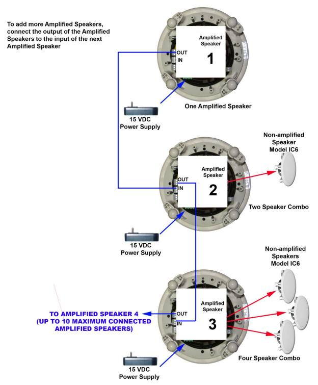
One, Two, Four Speaker Combination Wiring
