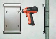
5. Mount the bracket on the wall using the four 3mm self-tapping screws.
