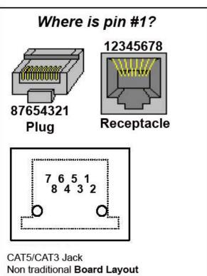
Note: The RJ-45 connector is on the component side. Shown here are the pins poking through from the component side of the board to the solder side of the board. But the connector pin-out is standard as pictured above.
