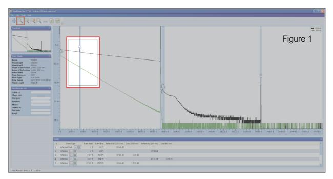
The highlighted rectangle in Figure 1 is a click-and-drag operation. Once the mouse button is released, the trace area changes to show the area of the trace produced by the rectangle (see Figure 2 below).
