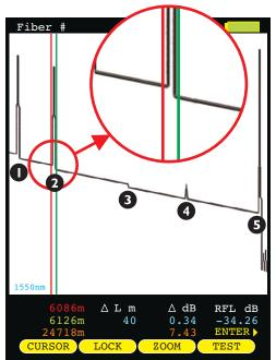
If the slope of the trace appears to "dip" to a lower level after the event (events 1, 2, and 3), this could mean one of two things: 1) if the slope of the line changes, the refractive index of the fiber preceding the
