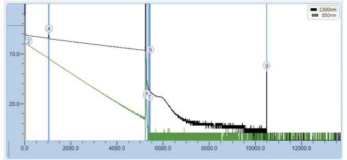
Power level. Shown in dB on the Y axis; 0 dB (a.k.a. origin) can be set to either top or bottom of Y axis.
