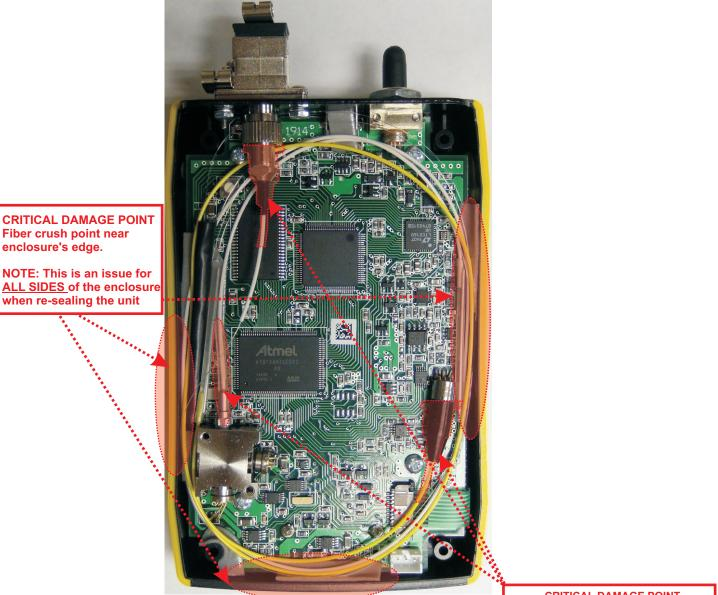
CRITICAL DAMAGE POINT Fiber coupling to laser and photodiode
