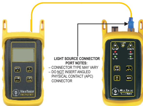
WaveSource connected to 1310nm port
