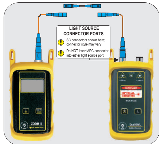
Insertion Loss Test
