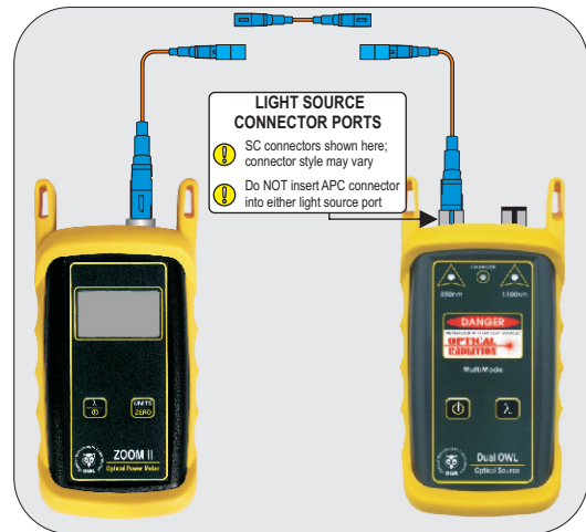
Insertion Loss Test
