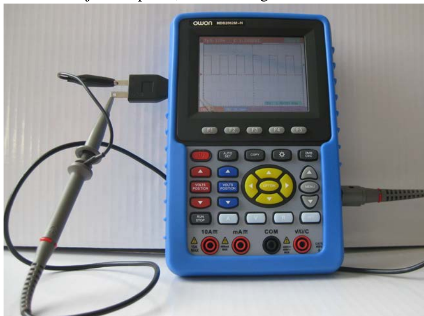
Fig.3. The connection of Square-wave test signal
