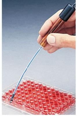
• Rugged Bulb Electrodes - more robust design to prevent breakage; great for field use
