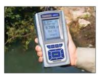
Rubber boot protects meter in rugged environments
