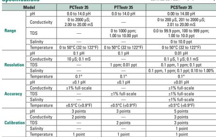
Temperature compensation: automatic (ATC), from 0 to 50°C (32 to 122°F) or manual
