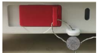
Locked with Wire Seal
