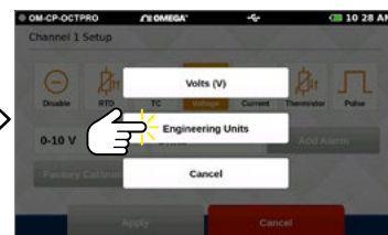
Select Engineering Units
